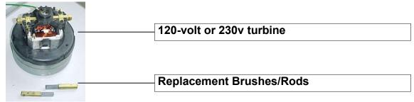
b) There are (2) rods on each motor and (2) Phillips screws holding down each rod.
