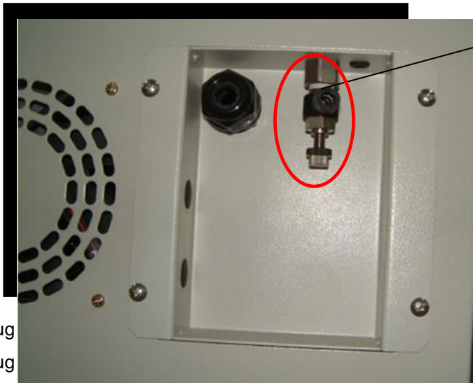
Air Assist Valve located at bottom right side for 100W models
