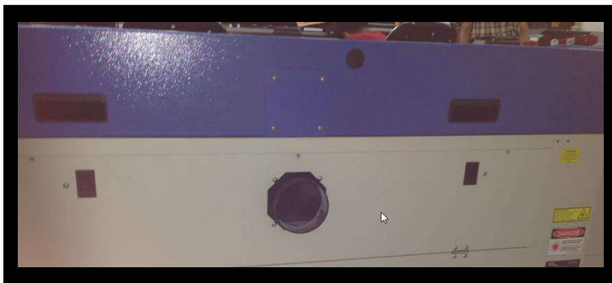
Remove screws securing rear door and exhaust duct
