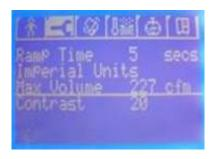
4.) Take note of the original/current value. Press the left arrow. The word calibrating appears in the lower left corner. The blower motor will run at the full speed, and determine the amount of air flow that is possible.
