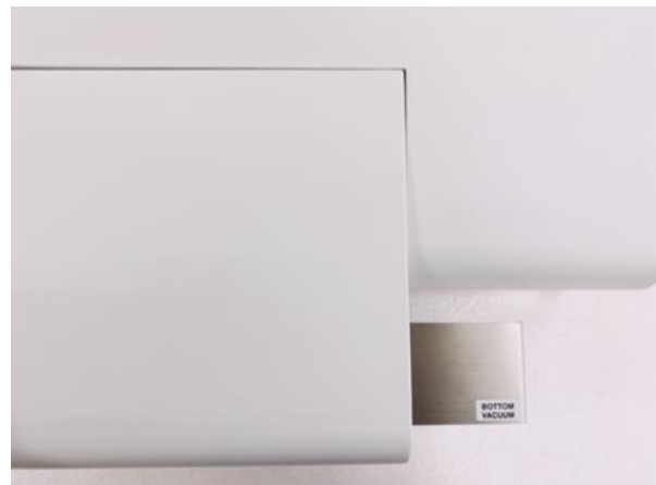
Pull the bar to the left side to increase the Bottom Vacuum
