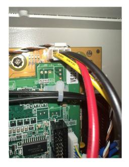
Unplug the power connector on main board. Switch ON the machine.
