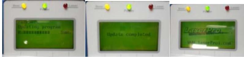
You will see status updates on the control panel of the machine. When the update is complete the machine will restart.
